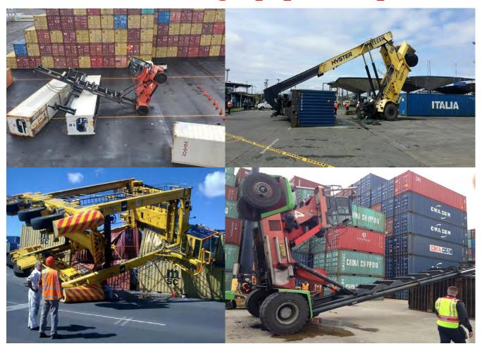
*From a global perspective*, the ILA~USMX Joint Safety Committee understands that tip-overs involving container handling equipment of the type shown above are occurring on a far too frequent basis lately. Those types of accidents are very dangerous and can result in serious/fatal injuries.
