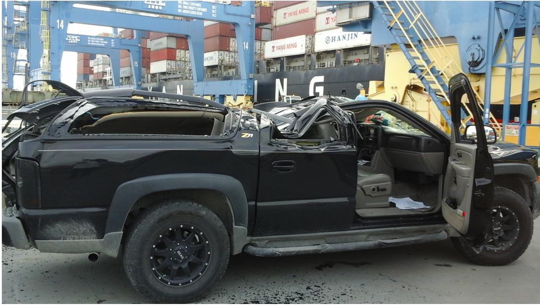
The photo above is of a marine terminal operator's company car that, on 26 March at a South Atlantic port, had a 40 ton hatchcover landed on it while temporarily parked in the backreach of a container crane. Two management representatives were occupying the front seat at the time. Incredibly, they escaped with only minor injuries. Obviously, this incident could have had a much more severe outcome.
